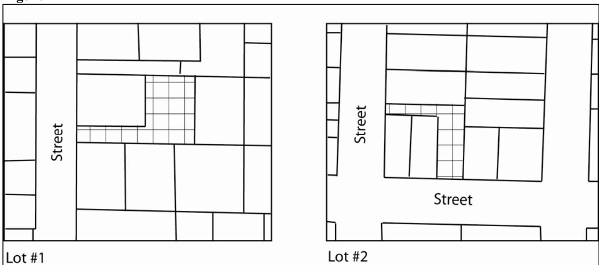
Two sample lots (shown with cross-hatching) with six sides in a typical “panhandle” shape.
